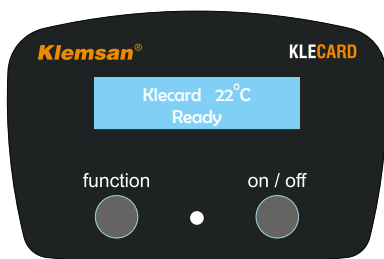
Printer Ready, Media is placed on the plate, The LED is illuminated
